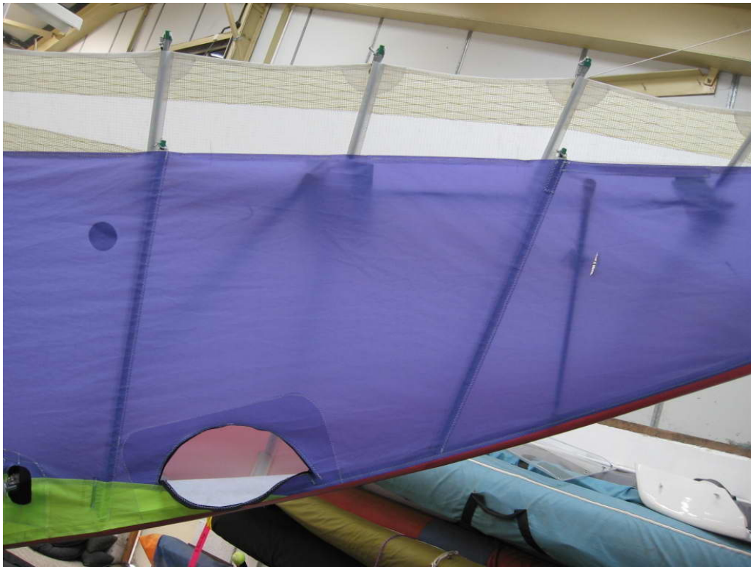
Rigging stage 12 – correct positioning of washout rods.
